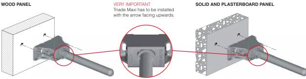
Recommended fixing pan head screw type - head Ø 5 mm max.
