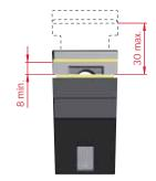
Shelf is clamped between a layer of ridged plastic on the lower side and soft rubber on the upper side (coloured parts).
