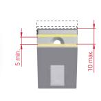
Shelf is clamped between a layer of white soft rubber on both the lower and upper side (coloured parts).
