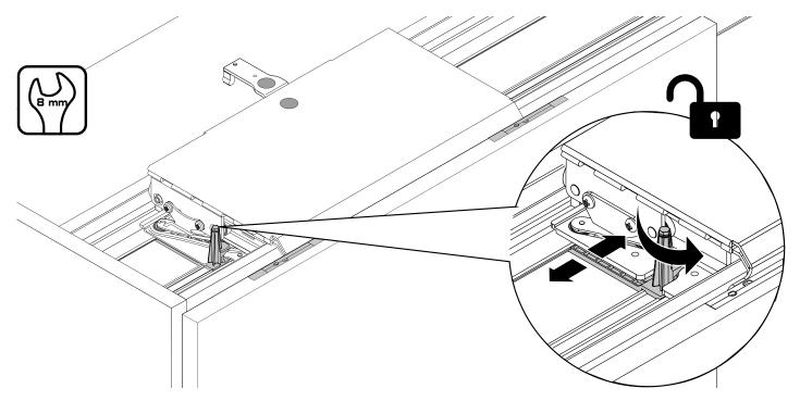
Check the vertical alignment and the central distance between the doors, eventually move the upper Left or Right locks.
