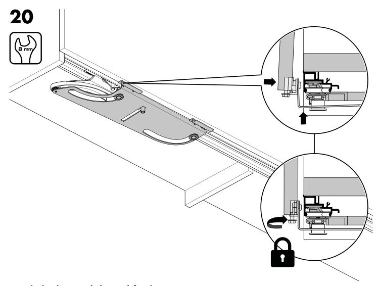
Hook the lower slide and fix the screws.
