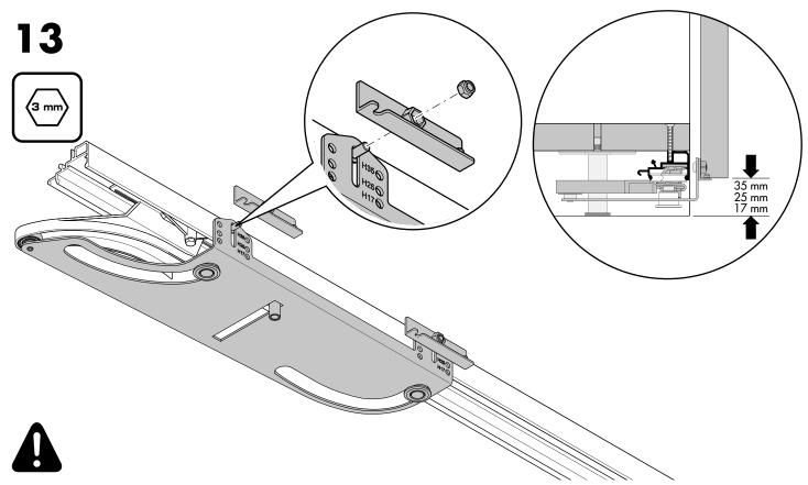
Distance between the door and the floor (17 mm, 25 mm, 35 mm).
