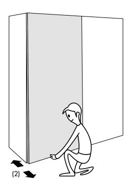
Slightly shake (2) the door at the bottom with both hands in this way the bottom stop will align automatically to the top stop. Lock the stops when finished.
