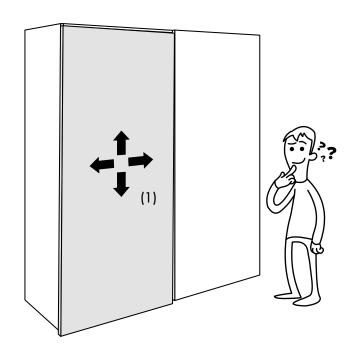
Do not forget to unlock the lower and upper stops before any further doors adjustment. (1)
