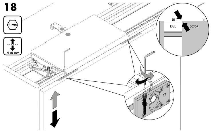
Close the door. Adjust the level of the door, aligning it with the upper rail.
